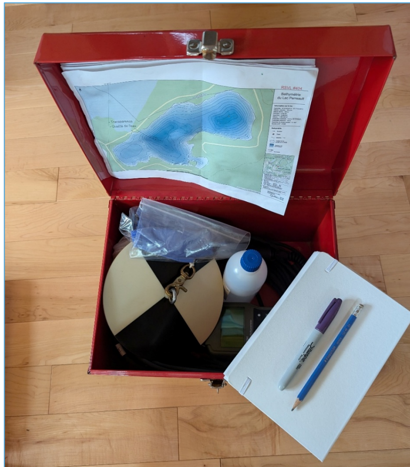
Figure 14: Example of a well-packed sampling toolbox. A backpack is also very acceptable, especially for river sampling. The box or backpack must be kept clean, organized, and be exclusively used for sampling materials. It should not be used to carry personal items, or food and beverages.
