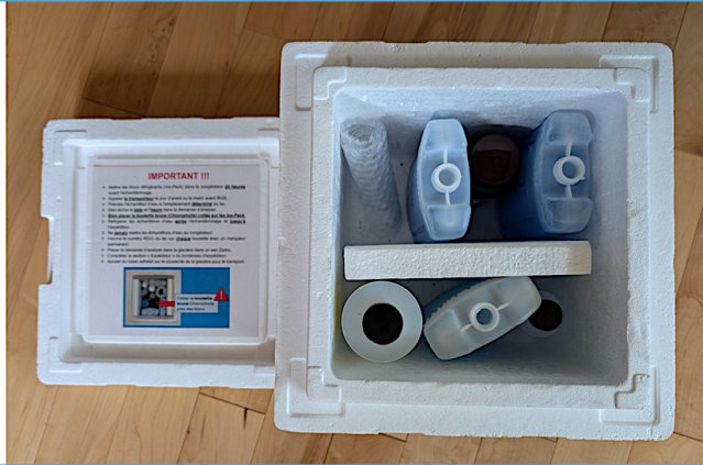
Figure 13: How to ensure optimal cooling conditions and safe transportation of sample bottles. Do not transport sampling tools and materials, personal items, or food or beverages in the cool box.
